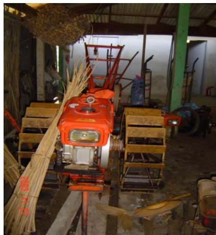
Figure 1 Diesel engine truck used for preparation of the cultivation field.
