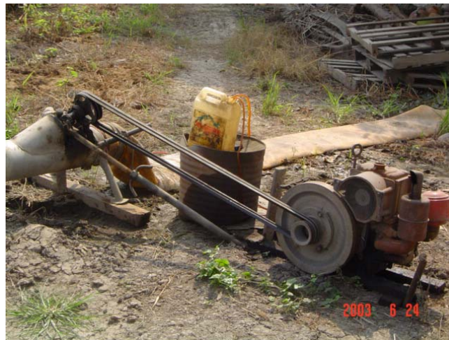
Figure 2 Diesel engine used for pumping water in and out the paddy-field.
